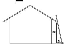
• Follow the manufacturer's instructors for placing the ladder at a safe angle. There should be no more than a 4:1 ratio between the height to the roof's edge and the distance from the eave. In
